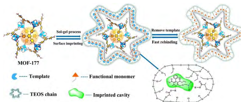
Figure 1. Fabrication of a core-shell sol-gel hybrid MIP based on MOFs.
